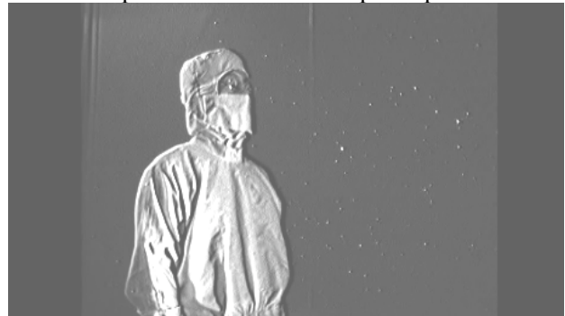
Fig.2 A cleanroom environment showing the airborne contaminant particles reflected in the laser light.
