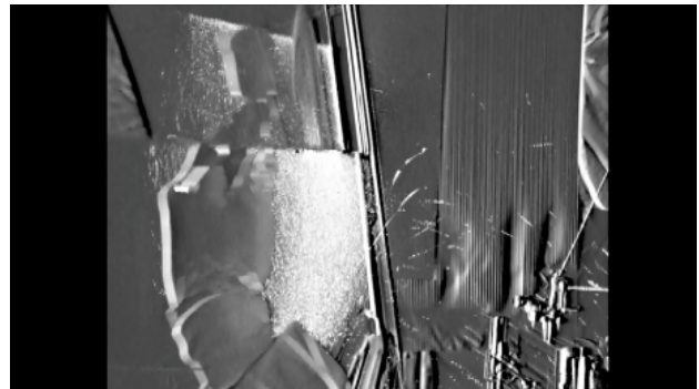
Fig.4 Time-lapse image showing particle concentration comparison across a test plane.
