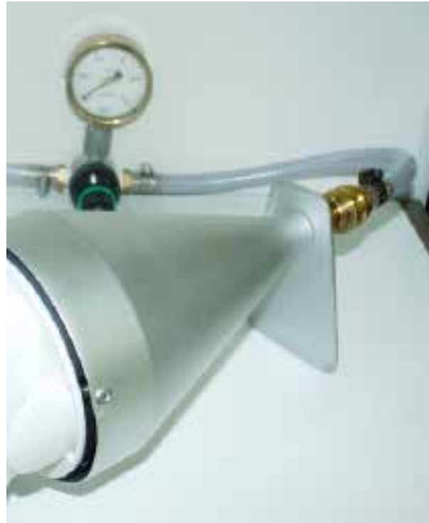
Fig1: Diffusor funnel (expansion takes place before collection, risk to damage microorganisms)
