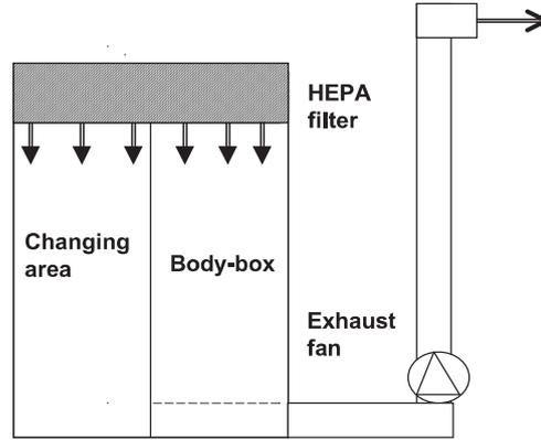
Figure 1 Principal arrangement of dispersal chamber (body-box).
