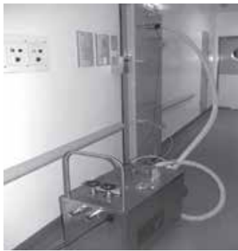
Air Leakage Test Rig photo courtesy of Clean Air Technologies
