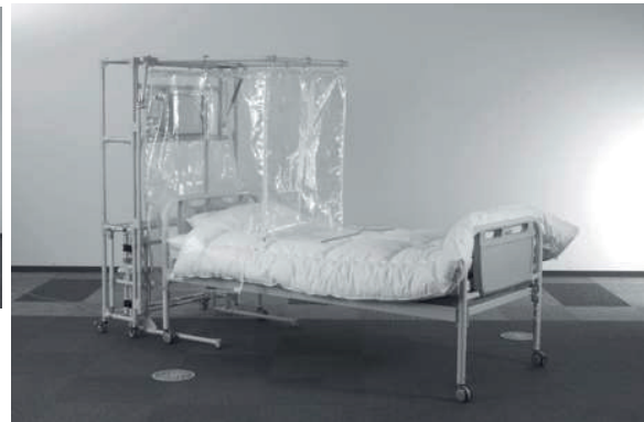
Figure 4 A bed equipped with the Barrihood for isolation of patients thought to have an airborne disease, such as pandemic influenza.
