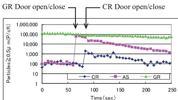
Fig.4 Particle concentration without clean-up cycle
