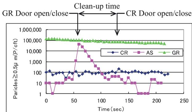
Fig.5 Particle concentration with clean-up cycle
