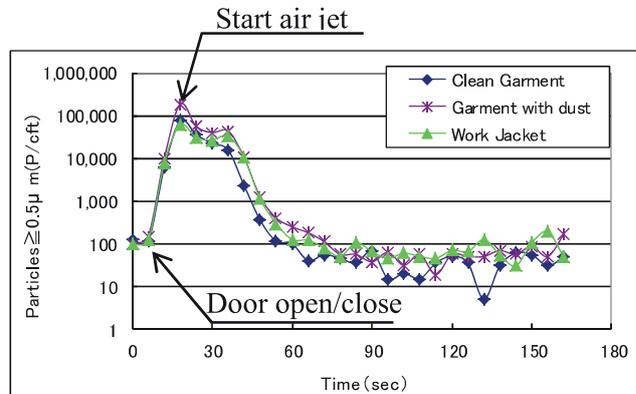
Fig.8 Comparison of particles generated by air jet from garments
