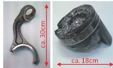
Figure 5. Damaged connection rod (left) and cylinder (right). Failure reason was a continuous gas injection caused by a micrometre sized particle.
