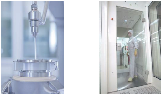
Figure 4. CO 2 snow cleaning as ultraprecision cleaning technology (left) used in the precision cleaning cleanroom at ESTEC (right).
